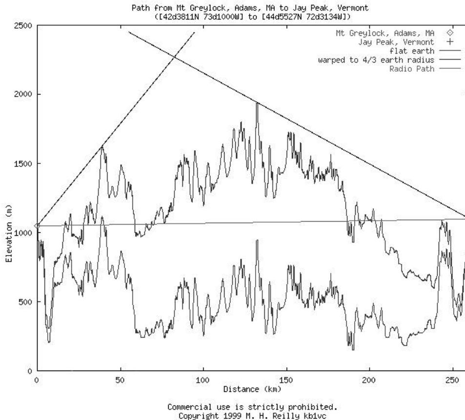
FIGURE 7 – Output From KB1VC Radio Line-of-Sight Path Plot Server
